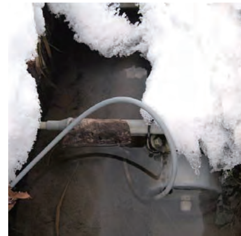
Motomiya : A turbidity meter and suspended sediment sampler at water-intake gate.
