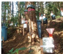
森林内の観測機器 (林内雨・樹幹流採取装置) Observation devices in a forest (Equipment for collecting throughfall and stemflow)
