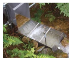
渓流水の流量観測 Stream water flow observation
