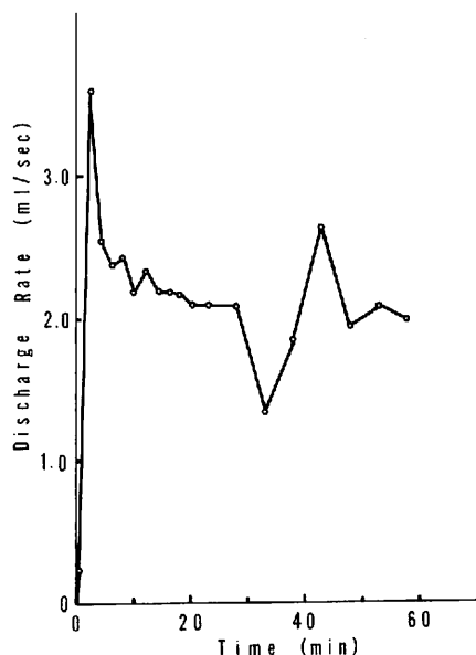
Fig. 3.4 Discharge hydrograph of the sand tank during the drying experiment.
