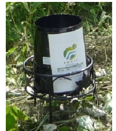
Measuring the precipitation and throughfall at multi-points.
