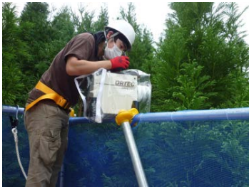
Radiation measurements using a portable Ge detector at forest tower
