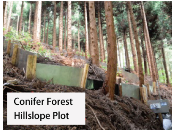
Measuring the precipitation and throughfall at multi-points.
