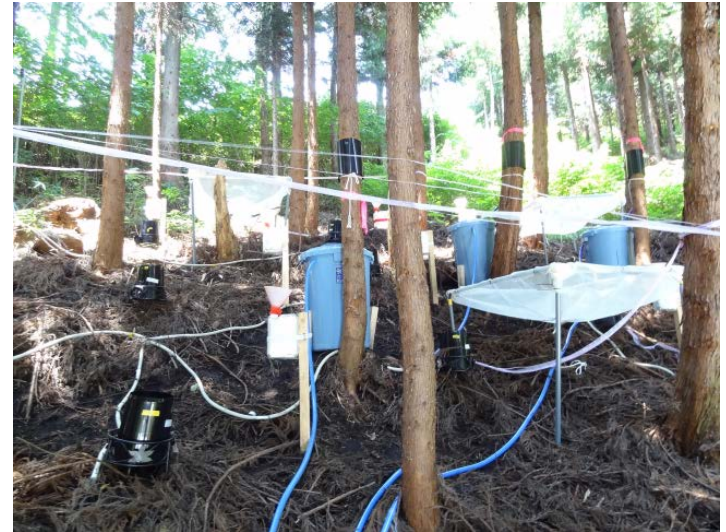
Measurement of stemflow, throughfall, and litter
