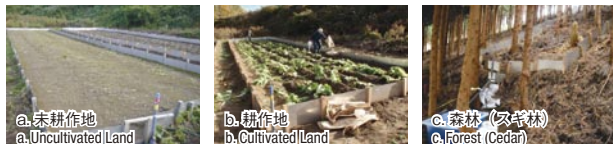
侵食区画からの土砂流出量の観測 Observation of soil erosion and sediment discharge volume from experimental plot
