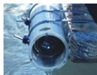
河川の濁度計測システム (河川水の濁り成分を計測) River turbidity measurement system (Measures turbidity component of river water)
