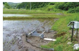
水田を介した放射性物質の流出モニタリング (量水堰及び濁度計測装置) Measuring discharge of radioactive substances through paddies (Flow gauging weirs and turbidity measurement equipment)
