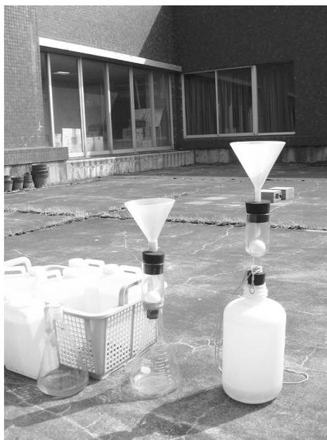
Photo 1 Precipitation sampler which have been settled at the rooftop of the Geoscience building, the University of Tsukuba
