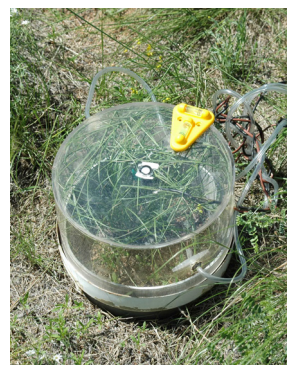
Fig 1 Measurement system Chambertop was made of acrylic resin, color was made of PV. Temperature sensor and PPF sensor were installed. 10 chambers were set on randomly.
